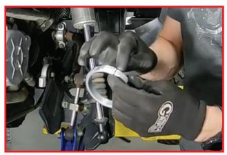
Starting at the bottom of the threaded shock body, rotate the cross over ring counter clockwise up the threaded shock body. Be careful not to cross thread and damage cross over ring or threaded shock body. Set cross over ring 6" from shock body cap. Do not tighten cross over ring, it will need to be moved once preload is set.
