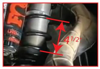
Align or clock lower coil end of new tender spring to upper coil end of new main spring. This reduces spring deflection.
