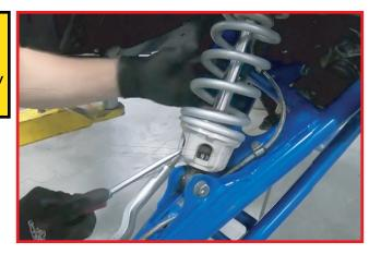
Loosen OEM upper preload ring from OEM lower preload ring. Use flathead screwdriver and hammer or mallet.
