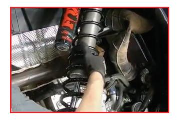
Set cross over ring by measuring 4 1/2" from top of spring divider. Then tighten cross over ring screws.
