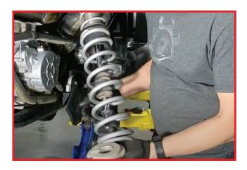
Install new rear billet cross over ring. Loosen the allen screws with a 3/32" allen wrench. Do not loosen allen screws all the way out.
