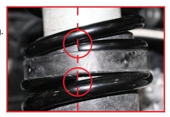
Positon cross over ring so that there is a 3/4" to 1" gap between bottom edge of cross over ring and top edge of spring divider. Tighten allen screws.
